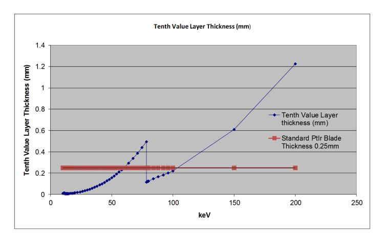
All Uniblitz XRS Series shutters come standard with platinum-iridium (PtIr) blades ("P" blades), allowing for a beam extinction of 90% at up to 30 keV x-ray energy.
