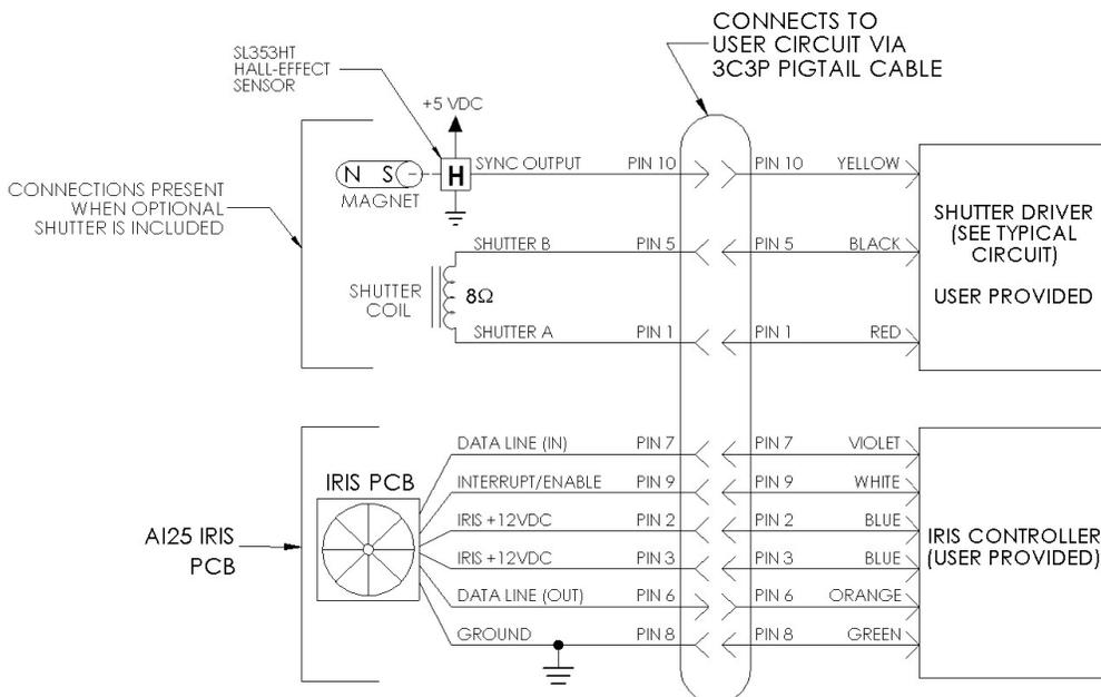
The AI25 schematic to the left depicts a device connected to user control circuits and the optional driver circuit through the 3C3P 3ft pigtail interconnect cable.
