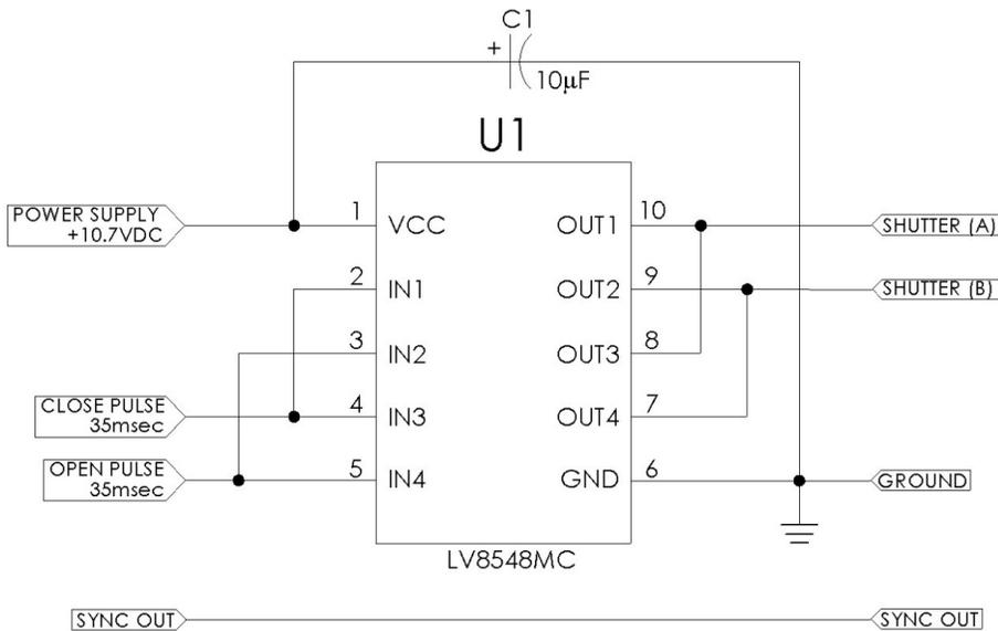
Sync signal can be a pass through as shown. The circuit to the left shows that 10.7VDC is supplied to the shutter driver circuit. If a voltage other than 10.7VDC is supplied, open and close pulse durations will need to be changed.
