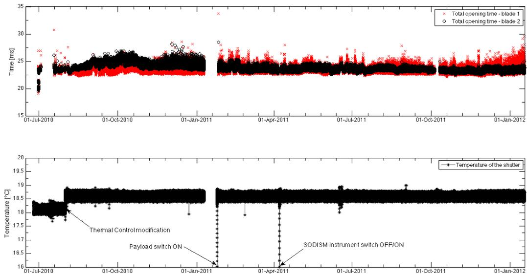
Figure 20. Evolution of total opening time and temperature of the shutter (in space).
