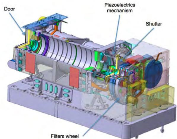
Figure 2. SODISM instrument.
