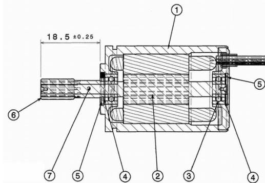
Figure 14. Stepper motor 1116112 (all dimensions in mm).
