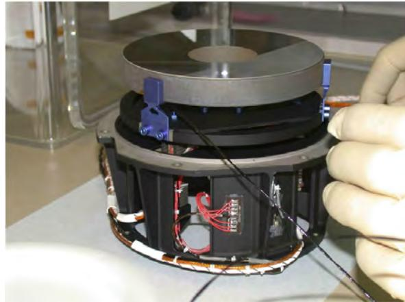
Figure 6. Qualification Model of the Pointing mechanism.
