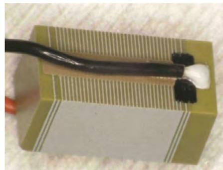
Figure 4. Standard multilayer piezoelectric component.
