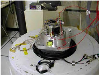
Figure 10. View of the Pointing Mechanism on the shaker.
