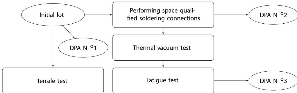
Figure 7. LAT test flow.
