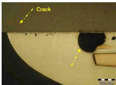
Figure 8. Cut of view of a soldering connection.
