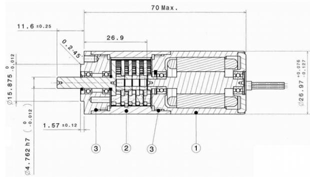
Figure 17. Stepper gear-motor 111611G1166A109.
