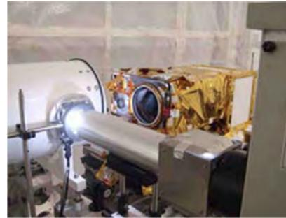
Figure 11. Test bench of SODISM instrument.
