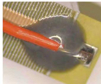
Figure 9. View of a soldering and secured connection.
