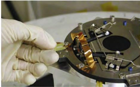
Figure 18. View of the SODISM electronic shutter.
