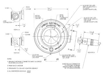
This drawing illustrates 6-pin connector and 1/4-20 threaded hole layout for the BDS25 series #3 housed style.
