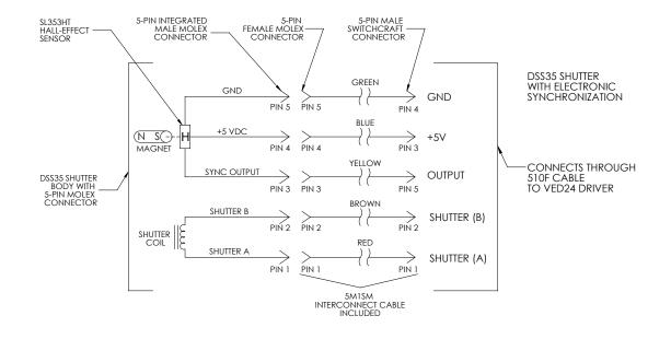
The synchronization system for DSS35B shutter devices incorporates a small magnet mounted to the driving mechanism and a Hall effect sensor. When the device achieves approximately 80% of full open, the magnet causes the Hall effect sensor to change state, producing a signal to indicate that the shutter has switched to the active state. Shown to the left is the DSS35B's shutter schematic which incorporates this electronic synchronization system.
